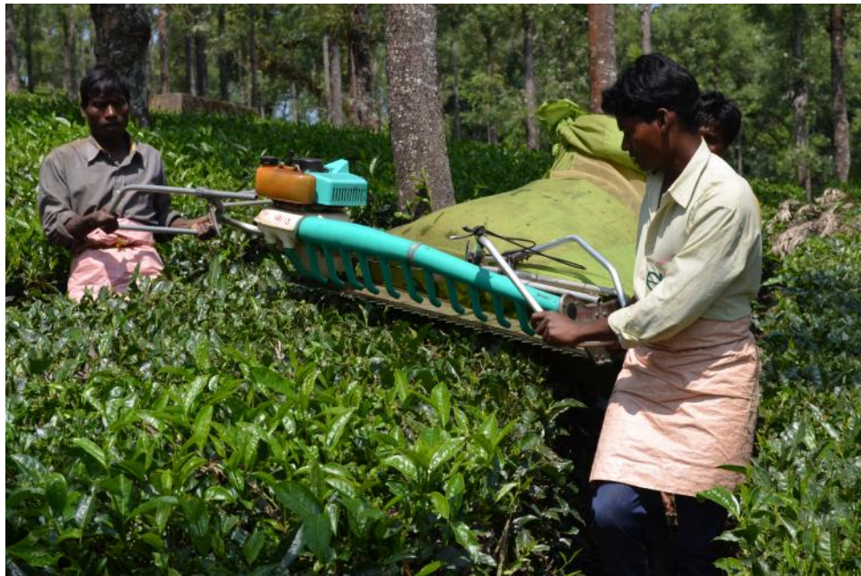
Two Men operated Tea harvester with 1.2m flat blade
